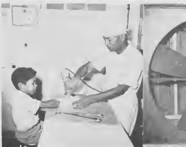
UNUSUAL AND not so unusual electric motor applications are pictured above. Fractional horsepower motors power a plaster cast cutter, above, and draftsmen's eraser, right. A much larger motor is needed to whirl the big four-foot Paint Shop fan, center.
